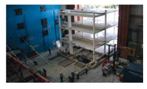
A 4-storey full scale model tested in the JRC's European Laboratory for Structural Assessment (ELSA) to study the effectiveness of seismic retrofitting of reinforced concrete frames.
